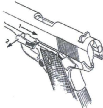
**FIGURE 7 REMOVING SLIDE STOP**
