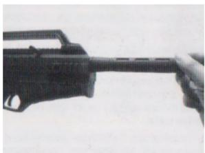
**27**- Screw the barrel cover clockwise.
