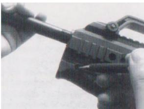
**15-** The assembly pim that you pushed. Stay in hole and it does not go out completely
