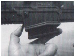
**6-** Release your magazine with the button which locates behind of the magazine
