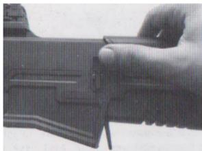
**10-** Push the mechanism release button on the left side of case.
