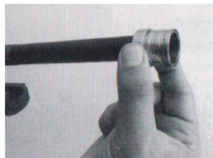
**22-** Assembly the piston as the picture that narrow side of the piston remains on the outside
